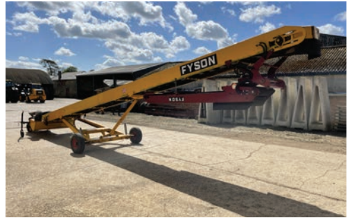
Fyson grain and potato elevator, approx. 10m, three phase electric, 415V motor, hydraulic control, hydraulic controlled swinging extension, transport wheels, tow hitch.
