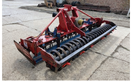
Lely Roterra 350 – 33 power harrow, 3.5m, rear coil press, rear levelling board.
