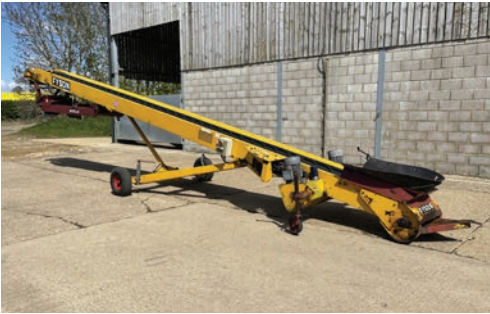
Fyson grain and potato elevator, approx. 10m, three phase electric, 415V motor, hydraulic control, hydraulic controlled swinging extension, transport wheels, tow hitch.
