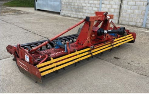
Lely Roterra 350 – 33 power harrow, 3.5m, rear coil press, rear levelling board.
