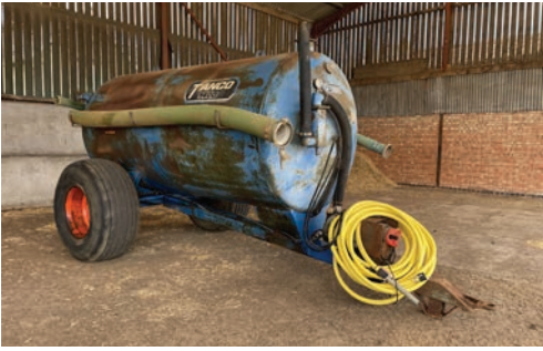
Tanco 1400 tanker, PTO pump, 4" and 6" outlets and hoses, 1.5" washdown hose, single axle, Goodyear tyres 550/60R22.5, s. no 1202.
