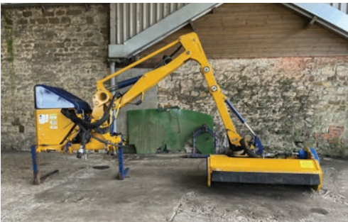
2007 Bomford Falcon 6T Parallel hedge cutter, telescopic arm, hydraulic lever controls, 3-point linkage frame mount, 2018 Bomford Turner Pro-Cut 1.6m flail cut head, hydraulic rear roller, LED lights, s. no B181835.
