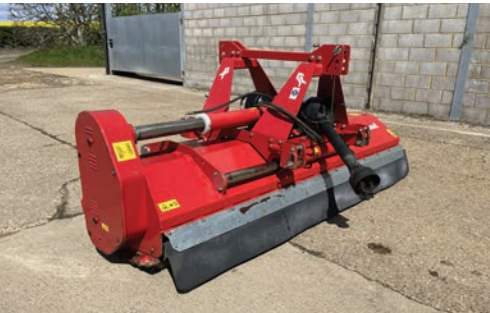
2011 Kverneland Macho FRO flail topper, 2.8m, front or rear mount, hydraulic side shift, roller, rubber skirt, s. no MACHOXX10117.
