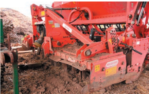
2012 Maschio Combi Orso 3000 power harrow, 3 metre working width, rear packer, s. no 1298R0279.
