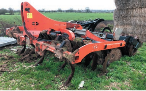
2013 Grégoire Besson Combi Mix one pass cultivator, five legs, two rows of discs, hydraulic depth controlled rear roller, 2.9 metre working width, 3 metre transport width, s. no N128991.
