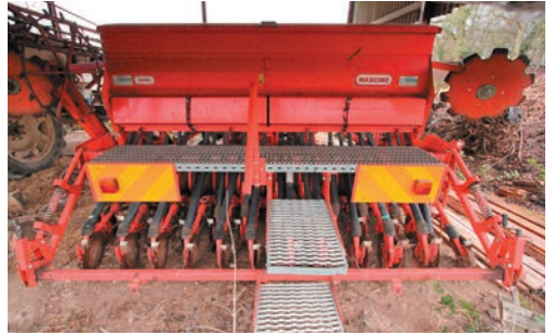
2012 Maschio DAMA 300 24DS DMRPK5 seed drill, 3 metre, disc coulters, trailing harrows, stand, s. no 129260247.
