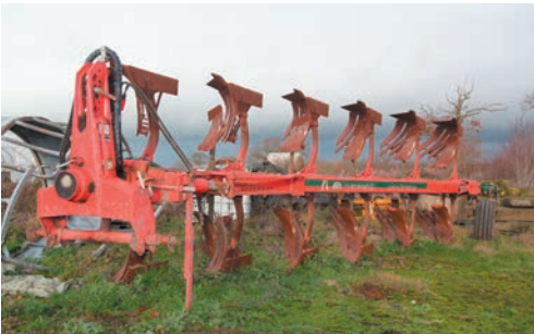
2010 Vogel & Noot Plus XS950 BA70 plough, six furrow, reversible, variable width, slatted boards, depth wheel, s. no 77388.
