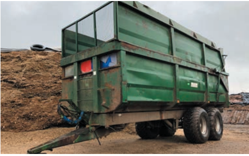
2003 Richard Western grain trailer, 16 tonne, tandem axle, c/w silage sides, hydraulic tipping, hydraulic rear door, sprung axles, sprung drawbar, hydraulic brakes, grain chute, flotation tyres, s. no 12289.
