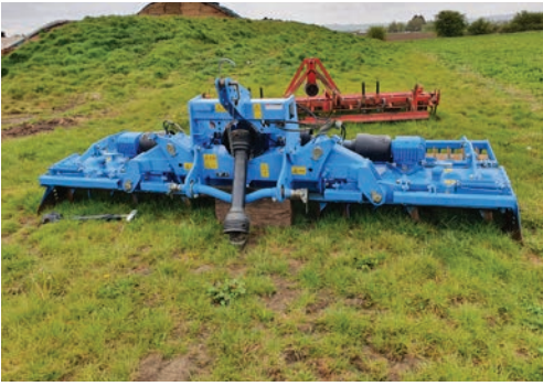
2017 Lemken Zirkon 12 power harrow, 4m, rear packer roller, hydraulic folding, s. no 441097.
