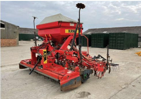
2009 KRM 300/25-R drill, 3m, 3-point linkage mounted, tine coulters, rear packer roller, trailing tine harrows, disc tramline markers, stand, s. no 48295, c/w 2009 KRM Magnum 300 power harrow, 3m, s. no 22894.
