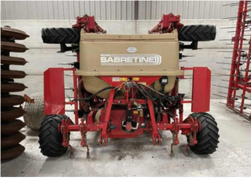
2014 Weaving Sabre Tine drill, 4.8m, 3-point linkage mounted, hydraulic folding, trailing tine harrows, disc tramline markers, LED lights, Stocks Ag Turbo Jet applicator, s. no 11018862.
