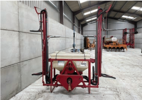
Horstine Farmery Microband avadex applicator, 12m, 3-point linkage mounted, land wheel drive.
