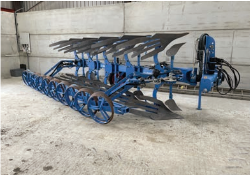
2018 Lemken Juwel 8 reversible plough, five furrow, slatted bodies, hydraulic vari-width, hydraulic land wheel, rear discs, skims, s. no 458627, c/w 2018 Lemken Flexpack JR5-100 press, s. no 458644.
