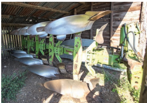
1996 Dowdeswell DP120S MA Delta Furra reversible plough, five furrow, land wheel, s no. MA36198.
