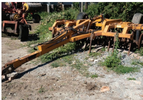
Simba double press, 3.5 metre, leading tines, trailed, hydraulic lift, s no. 40809072.
