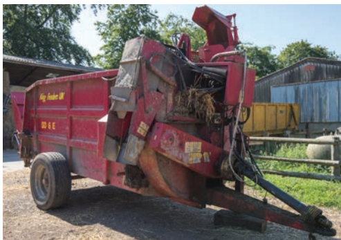
King Feeders UK SD 6 E straw chopper, PTO driven, single axle, electronic controls, hydraulic rear door.
