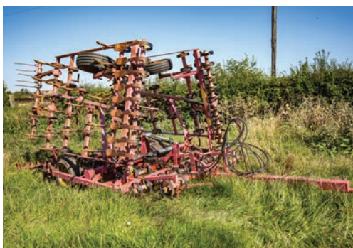
Vaderstad NZF Mark II tine harrows, 6 metre, trailed, hydraulic folding, levelling boards, tramline eradicators, s. no 13462.
