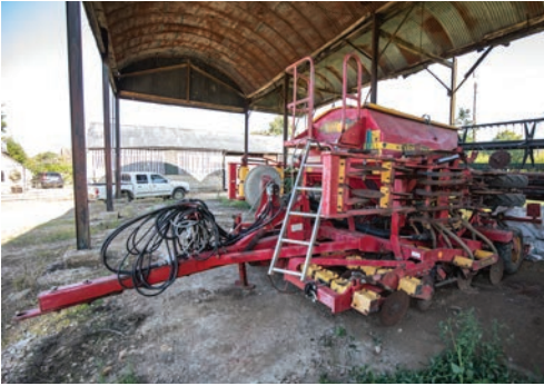
Vaderstad Rapid 400F disc drill, 4 metre, hydraulic folding, tine packer, one tonne hopper, tramline markers and trailing harrows, s. no 11189.
