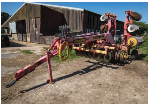
Vaderstad Carrier 425 discs, 4.25 metre, trailed, hydraulic folding, c/w Vaderstad Disc CR425 (s. no 2564), year – N, s no. carrier 0775K.
