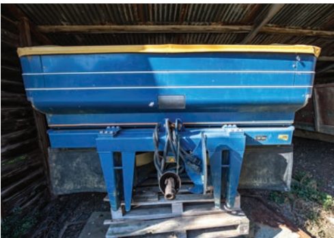
KRM M2W Q2 fertiliser spreader, 3-point linkage mounted, up to 24 metre spread, hopper cover, greedy boards, variable rate, electronic control box s. no 2498.
