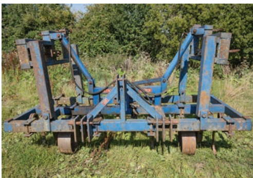
Blench pig tail tines, 4 metre, depth wheel, hydraulic folding, 3-point linkage mounted.
