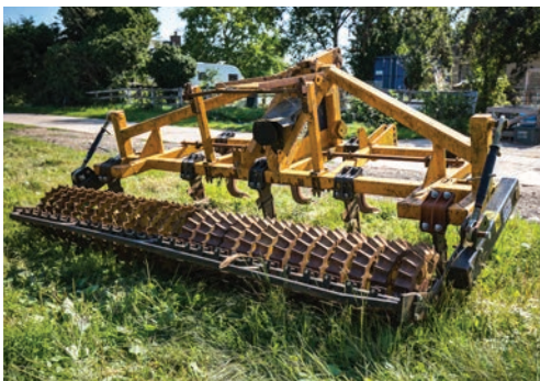
McConell Shakaerator , 7 leg, PTO driven, height adjustable rear press, 3-point linkage mounted, s. no 18CP29.
