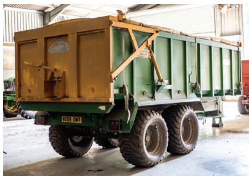
2009 Easterby ET12 grain trailer, 12 tonne, tandem axles, hydraulic brakes, suspended drawbar, leaf sprung axles, hydraulic rear door, grain chute, inspection ladder rollover sheet, Altura flotation tyres, s. no 4434.
