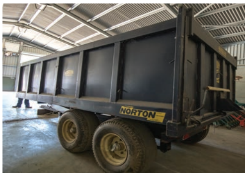
Norton grain trailer, 10 tonne, tandem axle, hydraulic tipping, leaf sprung axles, hydraulic brakes, manual rear door, grain chute, s. no 4816.
