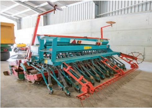
Reco Sulky Compact Master drill, 3 metre, disc markers, trailing harrows, land drive wheel, 3-point linkage mounted, hopper cover, s no. 94/cm09121.
