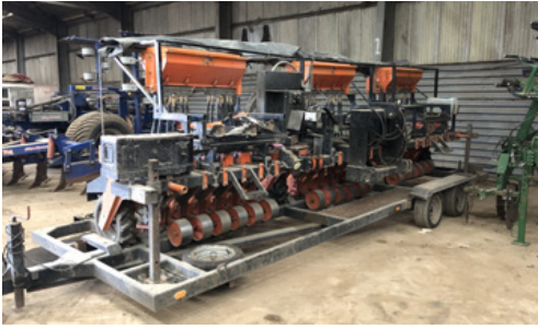
Stanhay carrot air drill, 3 x 2m beds, 12 row, 4" row, hydraulic fan, 3-point linkage mounted, c/w Vydate applicator kit, c/w canvass cover, c/w low loader transport trailer.
