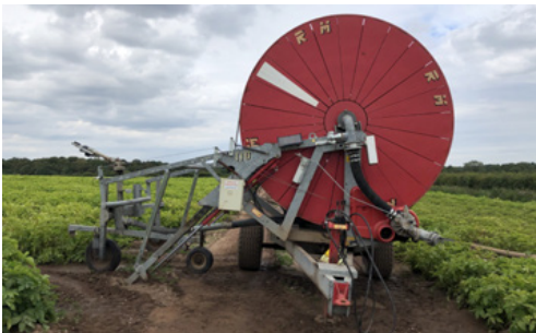
2010 RM Irrigation Super Rain 110/550 hose reel irrigator, 5,714 hours, 550m reel, 4" pipe, c/w Komet Twin 140 Plus galvanised adjustable rain gun, onboard computer, solar panel charge, hydraulic control, hydraulic turntable, machine type: 890 GX 110 550, s. no 890390.
