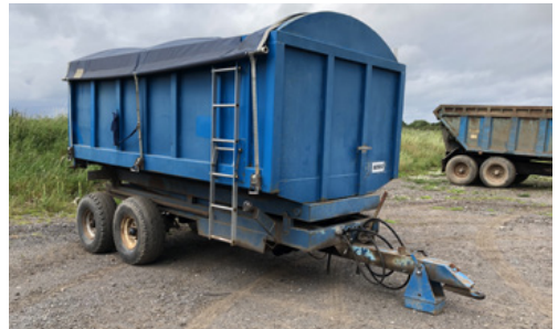
High tip scissor lift trailer, 6 tonne, tandem axle, hydraulic brakes, rollover sheet, twin grain chutes.
