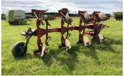
1996 Vogel and Noot Euromat Permanit 35 MS950 reversible plough, four furrow, manual variable-width, press arm, turf discs, manure skims, land wheel, s. no 033493.
