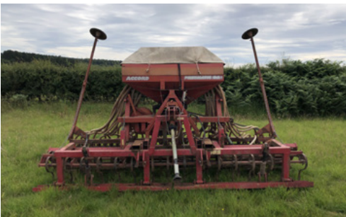
Accord Pneumatic DA air drill, 4m, Suffolk coulters, electronic tramlining, land wheels, disc markers, c/w Doublet-Record spring tines, crumbler roller, and levelling board.
