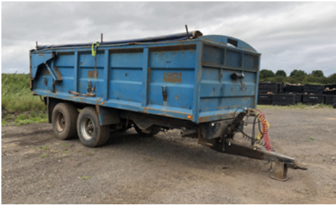
3 x AS Marston root trailer, 14 tonne, 10 stud commercial tandem axles, air over hydraulic brakes, hydraulic tipping, hydraulic rear door, leaf sprung axles, sprung drawbar, inspection ladder, super single wheels and tyres, grain chute, rollover sheet.
