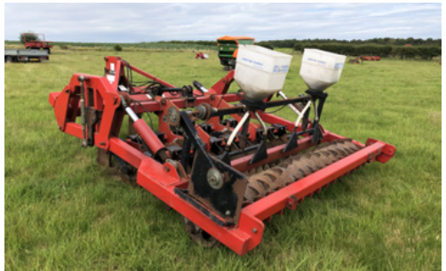
Spaldings 90/150 flat lift, 2.55m, three legs, s. no 900720, c/w Spaldings 12965 discs, s. no 2802585, c/w Spaldings 2288 hydraulic controlled rear packer roller, s. no 18213402, c/w Horstine Microband seeder.
