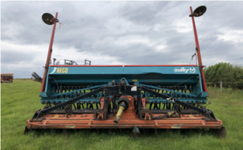
1989 Reco Sulky Compact Tramlines drill, 4m, Suffolk coulters, trailing tine harrows, disc markers, land wheel, s. no 93CT04104, stand, c/w Maschio 4000 power harrow, 4m, rear packer roller, s. no 826782.
