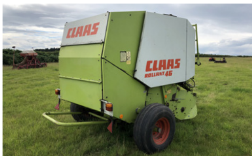
Claas Rollant 46 round baler, net and string, 4.52ft pick up reel, 540 PTO driven, electric control box, s. no 00702781HD.
