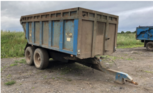
1988 Bailey dump trailer, 10 tonne, 8 stud tandem axles, hydraulic tipping, hydraulic brakes, s. no 1452.
