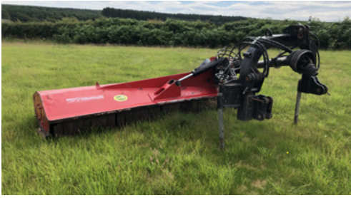
2015 Omarv SMI 260 E Big Cutter Off Set Professional flail topper, rear roller, 2.6m cut, s. no 090548.
