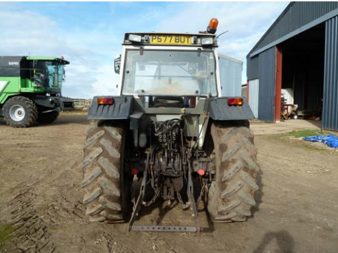
1997 Massey Ferguson 390 LoProfile+ 12/12 , registration P577 BUT, 4,318.72 hours, 4WD, c/w Massey Ferguson MF820 loader (s. no L1164), three manual spools, PUH, one former keeper, tyres 13.6R24 – 30%, 16.9R34 – 10%, s. no F10208.
