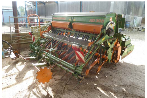
2008 Amazone AD 303 Special Vario-Control drill, 3 metre, Suffolk coulters, trailing tine harrows, tramline markers, land wheel, road lights, c/w polystyrene hopper divider, stand, s. no AD00031058.
