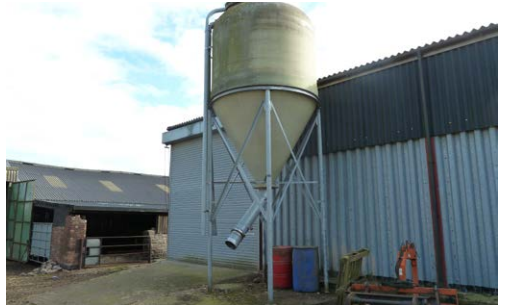
EB Equipment bulk feed silo, 8 tonne capacity.
