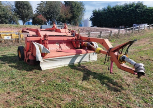
Taarup 338 B mower conditioner, 3m, hydraulic offset, trailed PTO driven, s. no 333771.
