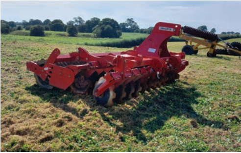
Proforge Inverta short disc harrow cultivator, 3m, 3-point linkage mounted, 22in cut away discs, steel packer, s. no 2961.
