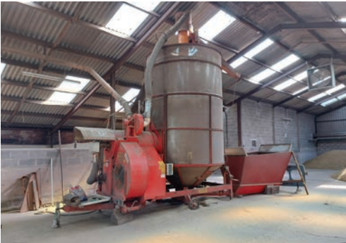
2003 Master Driers Junior 100E batch grain drier, ten tonne capacity, kerosene, electric control box, trailed, c/w hopper, s. no NE1603.
