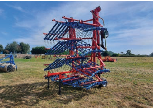
2016 Opico Grass Harrow , 12m, 7mm tines, hydraulic folding, scissor folding, 3-point linkage mounted, s. no 0188/16.
