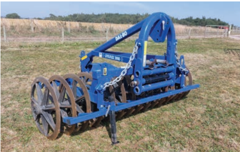
2011 Dalbo Levelflex 2008 front press, 3m, 3-point linkage mounted, c/w stand, s. no 02608.
