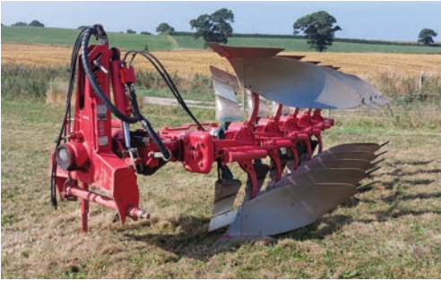
Vogel & Noot c-plus XS950 ST Vario reversible plough, five furrow, rear discs, skims, land wheel, type: C59C565A79, s. no 79265.
