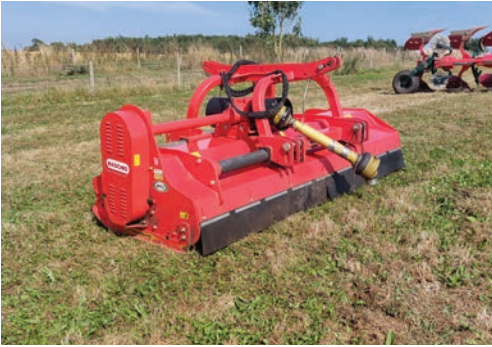
2020 Maschio Bufalo 280 heavy duty flail topper, 2.8m, front or rear 3-point linkage mounted, PTO driven, hydraulic side shift, rear roller, s. no KM91F0431.
